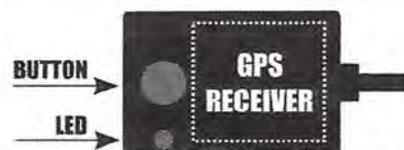
Place the receiver module with the writing facing upwards and in a horizontal position with a clear and unobstructed view of the sky placed in a way that pushing the button you will not cover the GPS receiver with your hand (see the image below); we suggest the fork plate of the bike or the top side of the dashboard.
